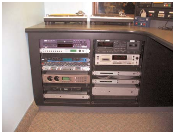
Along with the microphone processors, telephone hybrids and switchers, do not forget the delay unit and accessible “dump” button.
