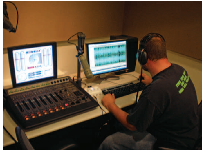
A UNLV student practices audio production in one of the edit booths using Adobe Audition. M!ka arms, Axia board and EV RE20 mics visible.
