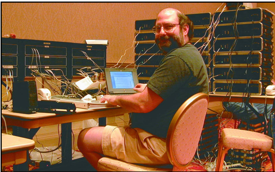
Barry Victor, director of engineering for the Radio Music Awards remote broadcasts, sits at the temporary Telos Zephyr farm during ISDN line checkouts. This farm eventually was divided and moved to rooms that were set up later.
