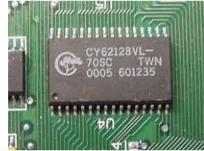
Picture of affected SRAM chip
