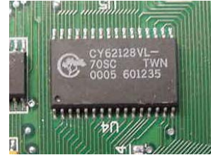
Picture of affected SRAM chip
