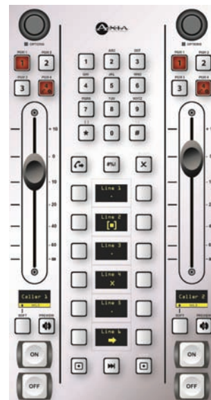
Figure 6: Mixing consoles integrate smoothly into an IP-based on-air telephone system. A single RJ-45 connects the control surface to both the mixing engine and telephone system. A telephone controller module allows convenient line selection and fader assignment at the talent operating position.
