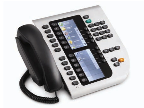
Figure 5: A desktop controller for an IP-based studio system connects via Ethernet. The large LCDs convey caller information entered into a PC-hosted producer application.
