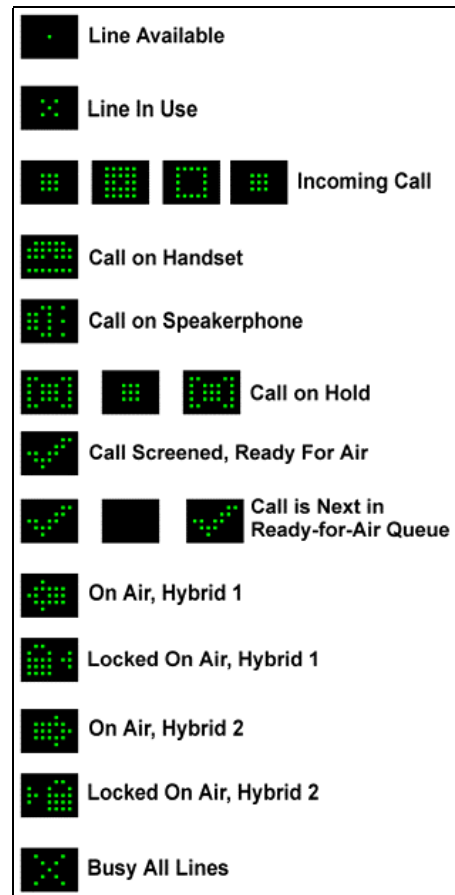
Fig. 4: An LED matrix display in the studio director phone can convey line status information more clearly than the usual blinking LEDs. Some icons may be enhanced with animation.
