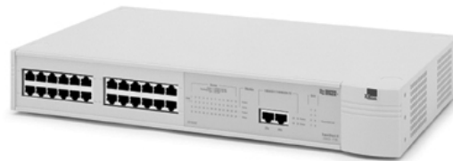
A “Stackable” Ethernet switch.
